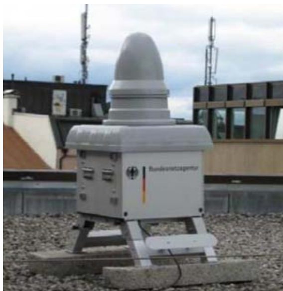
Slika 5.12 - Senzor Rohde & Schwarz EMF-Monitor
